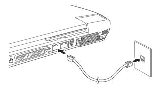
Figure 4-12 Connecting the internal modem
